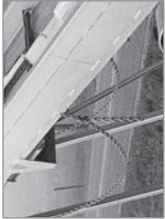
Safety Chain Securing Hooks-Left Side (TW-C30HD)
