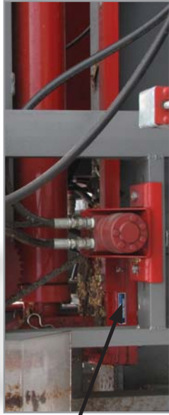
Shown Here: Splitter Cylinder Base
