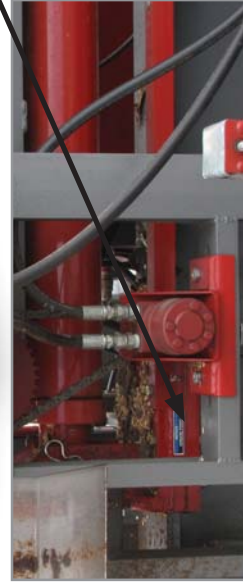
Shown Here: Splitter Cylinder Base
